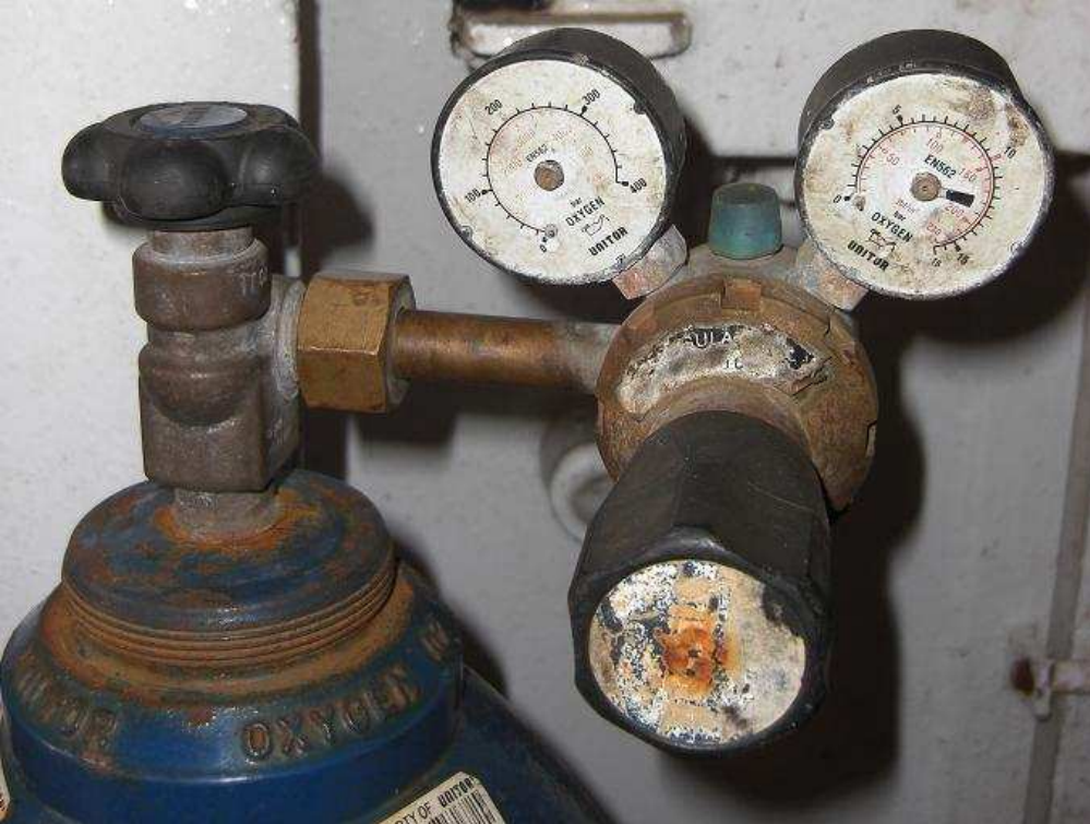
MV MSC Rebecca: hatch accesses not watertight closable, gas welding equipment and piping wasted, etc.
