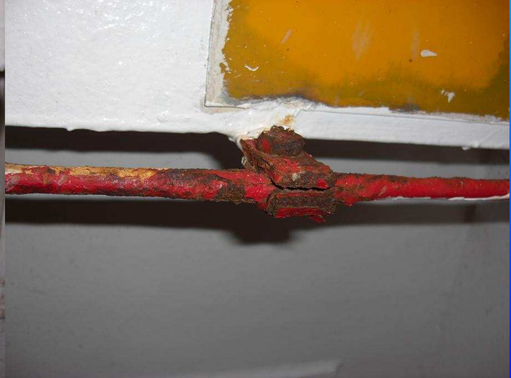
MV MSC Rebecca: hatch accesses not watertight closable, gas welding equipment and piping wasted, etc.
